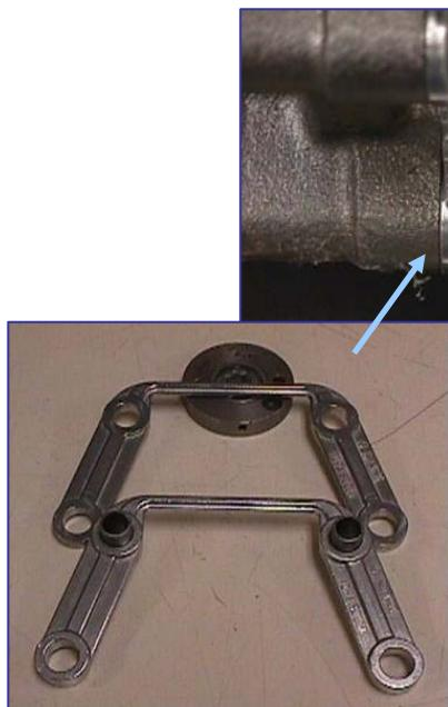
Figure 1 – Power Steering Pump Spacer. On the left, a machined prototype is adjacent to a die casting component. Above, a die casting assembled to the pump.
